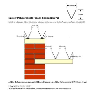
Narrow Polycarbonate Pigeon Spike (BS370) Rod Material: UV stabilised polycarbonate Base Material: UV stabilised polycarbonate
